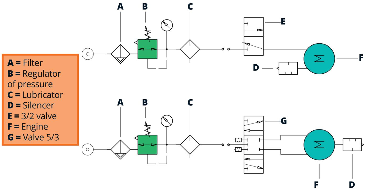
**Non-reversible motor operation with 5/3 closed-center valve**
